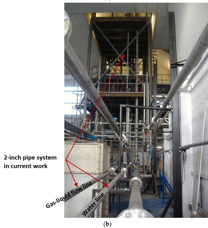
Figure 1. (a) Schematic of the test facility at Cranfield University. Images in insets shows the WMS used and circumferential air inlet for the riser base injection. The variable D is the internal pipeline diameter. (b) Actual photo of 52 mm experimental facility.
