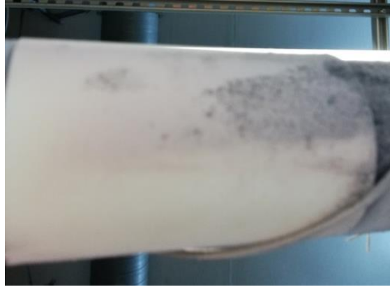
Figure 6-60: Downstream of the ceramic probe n°3 (~ 600°C, d_t = 39 mm) after 5 hours from combustion of Daw Mill-12 wt.% Miscanthus using the 2 nd probes' configuration.
