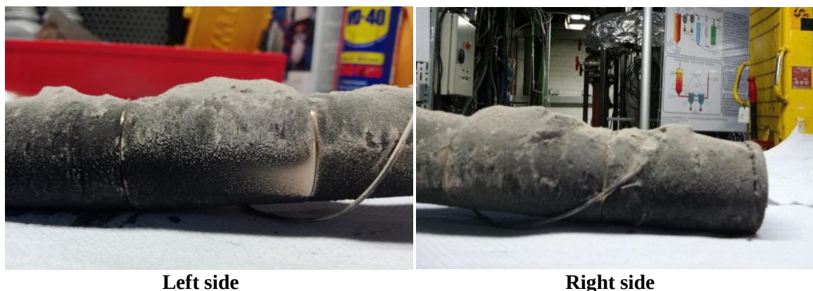
Figure 6-20: Deposit formed on probe 3 ( \sim 500^{\circ}\text{C} , d_t = 39\text{ mm} ) after 5 hours from combustion of Daw Mill-12 wt.% Miscanthus using the 1 st probes' configuration.
