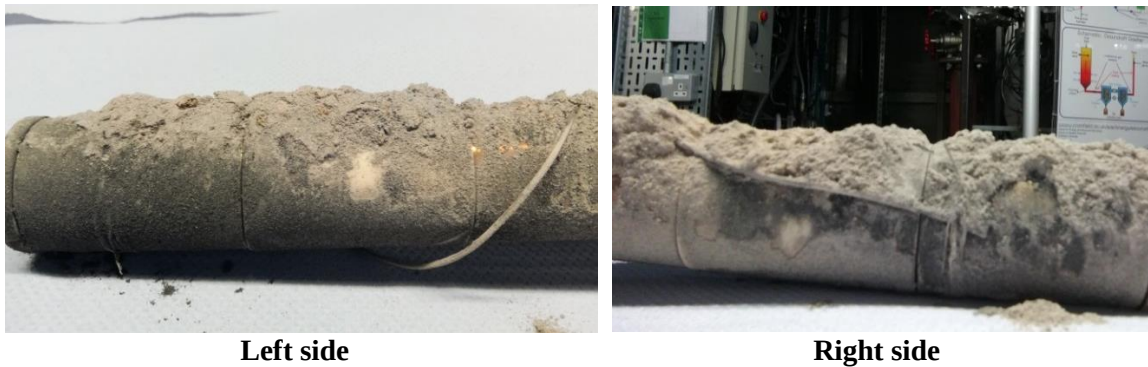
Figure 6-39: Deposit formed on probe 2 ( \sim 500^{\circ}\text{C} , d_t = 39 mm) after 5 hours from combustion of Daw Mill-12 wt.% Miscanthus using the 2 nd probes' configuration.
