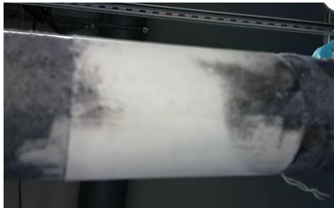
Figure 6-6: Downstream of the ceramic probe 1 ( \sim 500^{\circ}\text{C} , d_t = 39 mm) after 2.5 hours from combustion of Daw Mill-12 wt.% Miscanthus using the 1 st probes' configuration.
