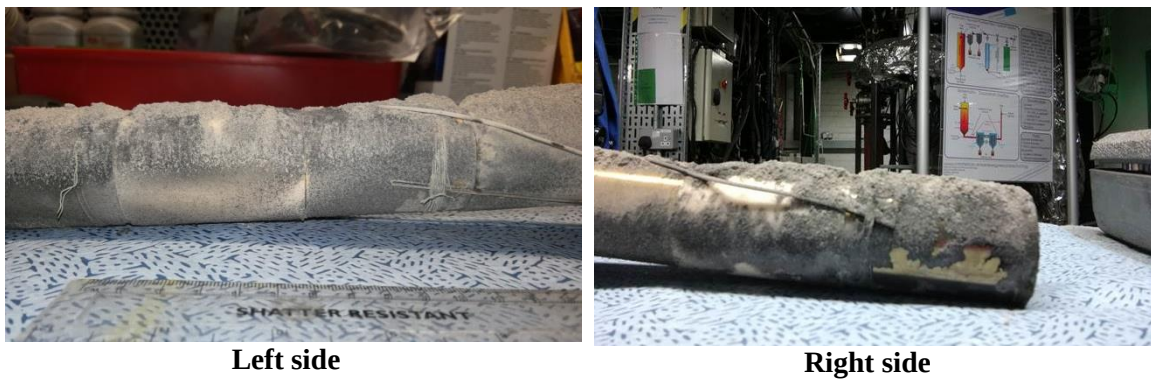
Figure 6-5: Deposit formed on probe 1 ( \sim 500^{\circ}\text{C} , tube diameter, d_t = 39 mm) after 2.5 hours from combustion of Daw Mill-12 wt.% Miscanthus using the 1 st probes' configuration.
