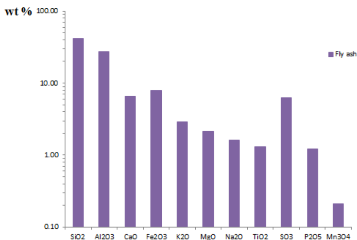
Figure 6-69: Average chemical composition from fly ash collected from the ports 1, 2 and 3 after 5 hours from combustion of Daw Mill-12 wt.% Miscanthus using the 2 nd probes' configuration at ~ 600°C (in terms of highest oxides of elements).
