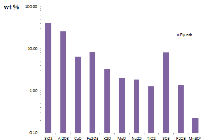
Figure 6-29: Average chemical composition of fly ash collected from the ports 1, 2 and 3 after 5 hours from combustion of Daw Mill-12 wt.% Miscanthus using the 1 st probes' configuration at ~ 500°C (in terms of highest oxides of elements).
