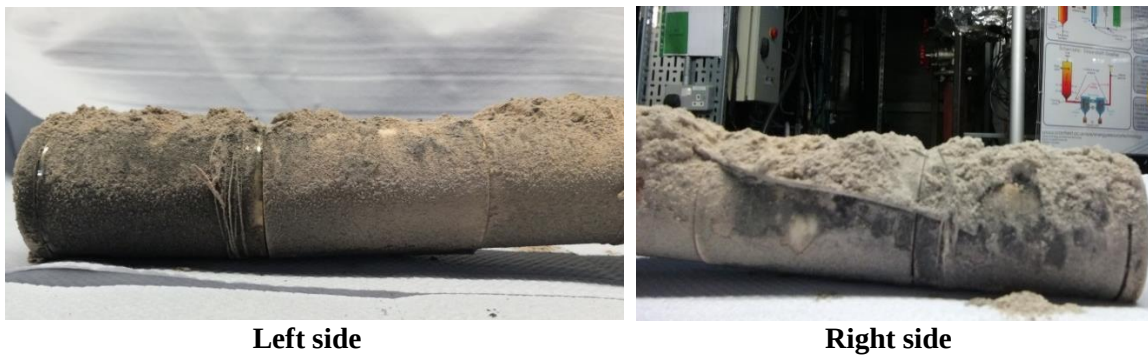
Figure 6-38: Deposit formed on probe 1 ( \sim 500^{\circ}\text{C} , d_t = 39 mm) after 5 hours from combustion of Daw Mill-12 wt.% Miscanthus using the 2 nd probes' configuration.
