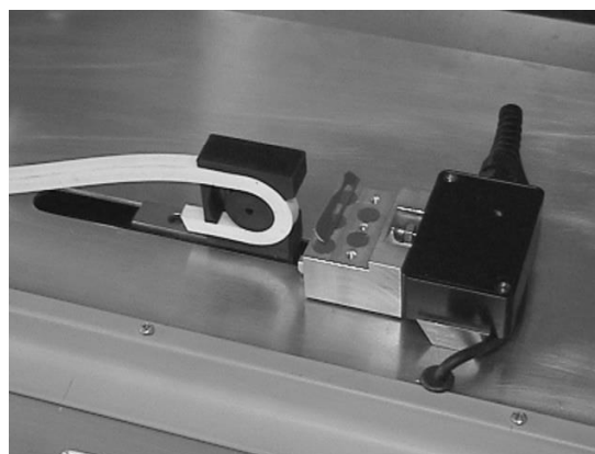
Figure 9. CATRA prototype sharpness measurement machine
