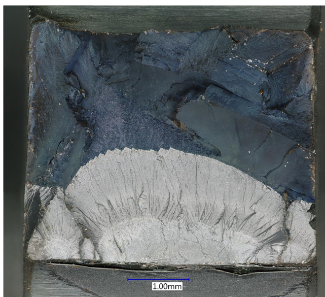
Fig. 16 | An optical image showing the crack surface morphology upon complete failure of the CMSX-4 fatigue specimen after 1505 cycles.
