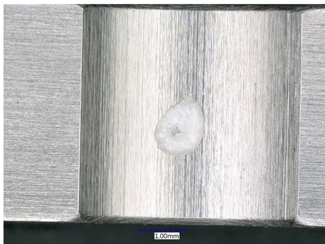
Fig. 15 | An optical image to show the singular droplet of salt solution being placed at a central point along the notch of a CMSX-4 fatigue specimen.
