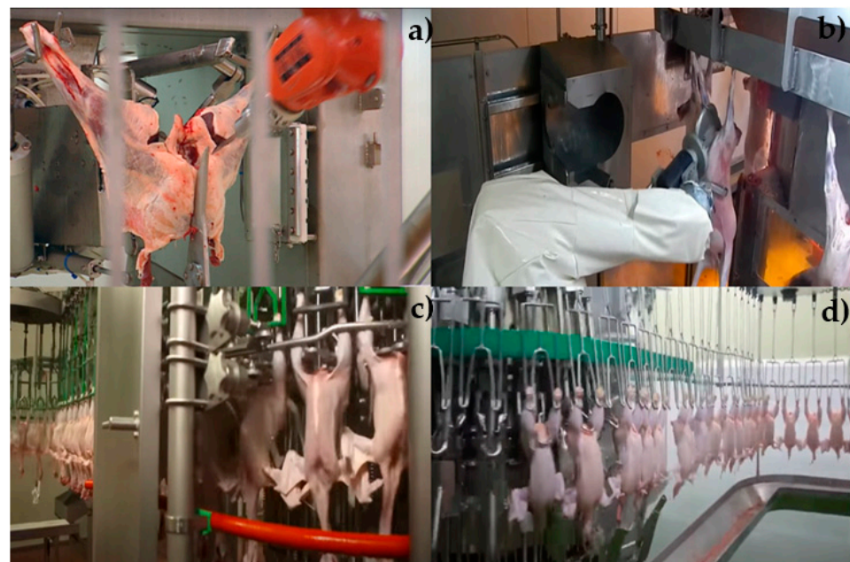
Figure 3. Robotics and automation in the meat sector ((a) bovine hindquarter cut; (b) lamb ventral cut; (c,d) automated poultry line).
