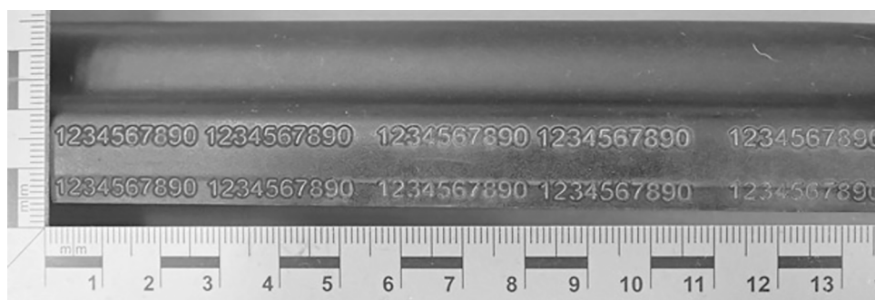
Fig. 3. The left side of an AK-pattern rifle top cover, with ten laser engraved marks (“1234567890”).
