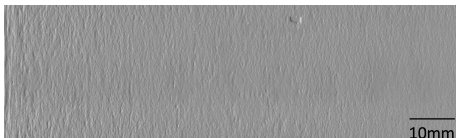
Fig. 5. The clearest magneto-optical image of the obliterated steel plate microstructure.
