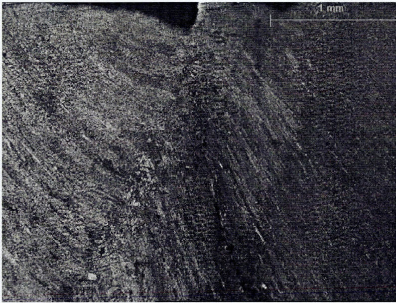
Figure 119: IIIS4M0325. Upper portion of a crack.
