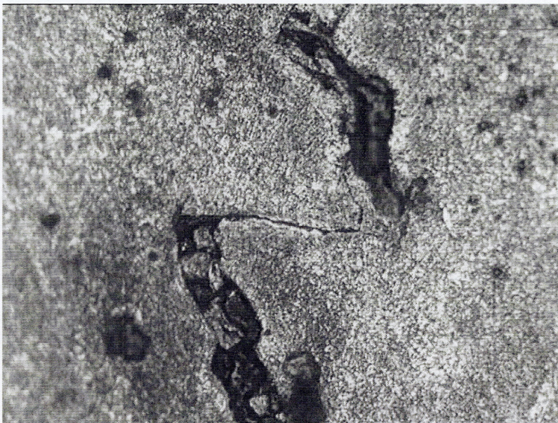
Figure 120: IIIS4M0325. Detail of a two cracking portions linked by a smaller crack.
