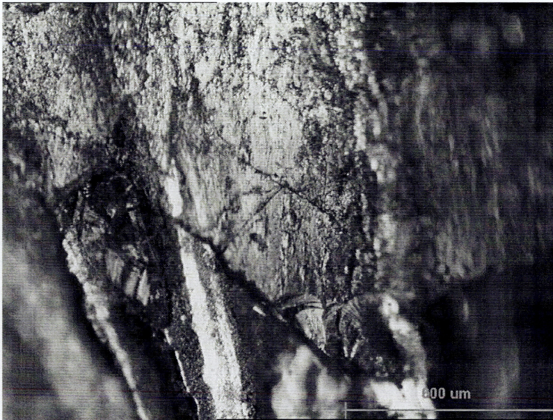
Figure 133: IVS6M0630. Detail of a surface crack.
