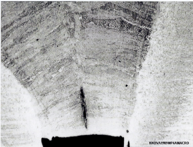
Figure 122: IVS4M0325. Centre-line solidification crack.
