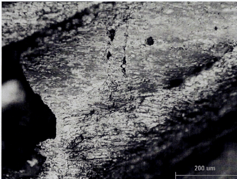
Figure 132: IVS6M0630. Detail of a surface crack.
