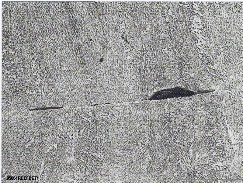
Figure 98: IIIS1M0325. Transverse cutting, sample 4R. WM defect.
