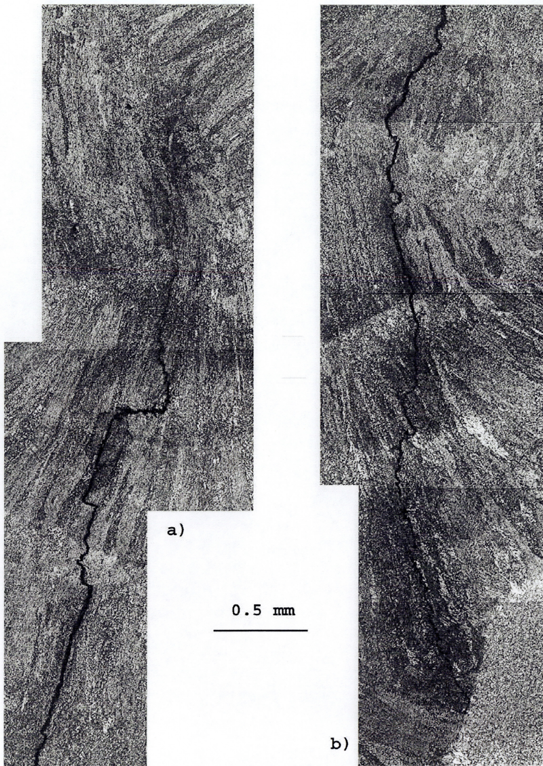
Figure 94: IIIS1MO325 – Sample 1F – Cracking extension – a) Upper and b) lower portions.
