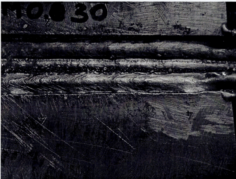
Figure 136: IXS6M0630. Macro-view of the weld surface.
