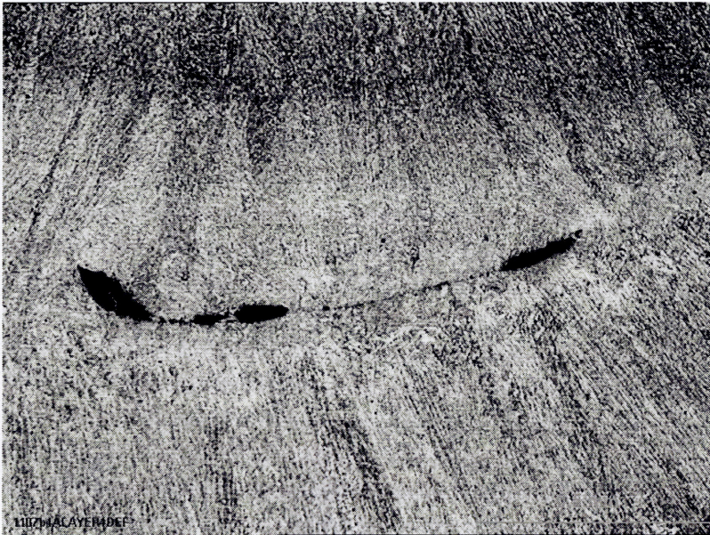
Figure 88: VIS1M0325. Weld metal defect.
