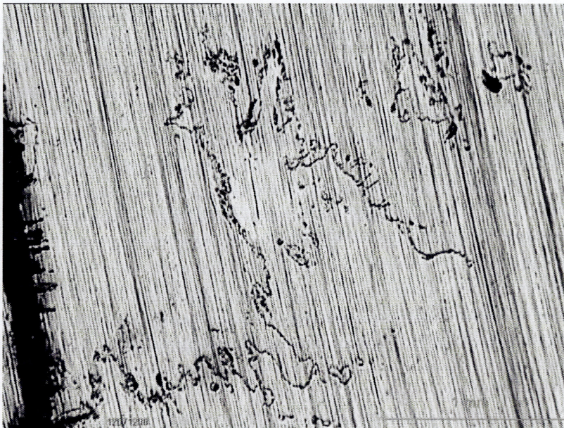
Figure 104: IXS1M0325. Small cracking connected to main longitudinal cracking. Unetched sample.
