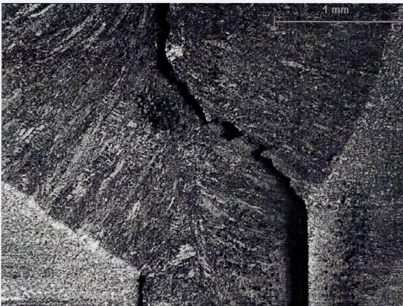
Figure 118: IIIIS4M0325. Macro-view of a cracked transverse section.
