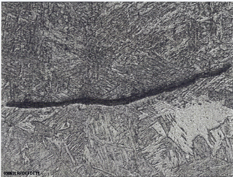
Figure 100: IIIS1M0325. Longitudinal cutting, sample 3L. Root pass defect.
