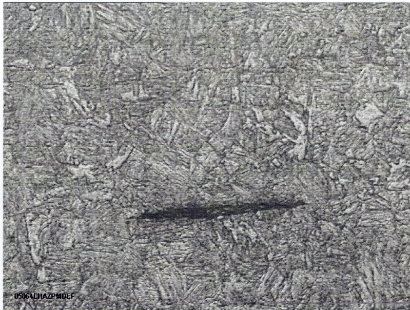
Figure 97: IIIS1M0325. Longitudinal cutting, sample 4L. HAZ defect.
