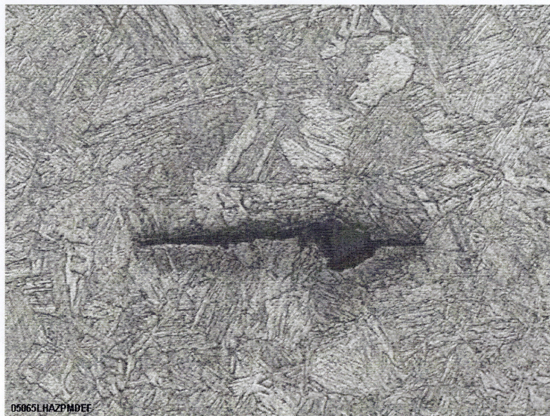
Figure 96: IIIS1M0325. Longitudinal cutting, sample 5L. HAZ defect.
