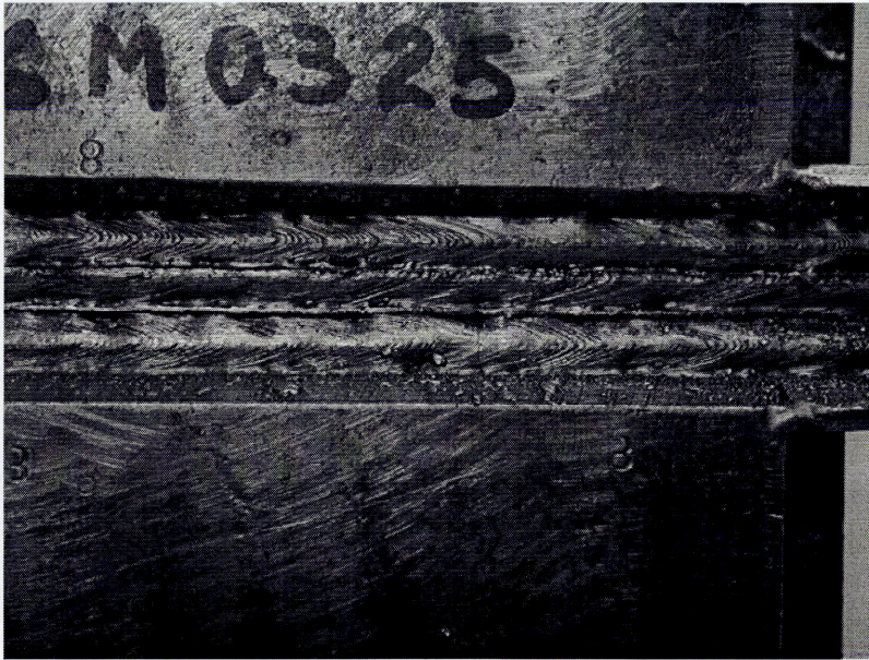
Figure 135: IXS6M0325. Macro-view of weld surface.
