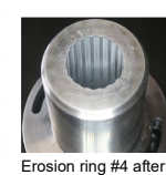
Erosion ring #4 after firing 50 shots with propellant 387A1.
