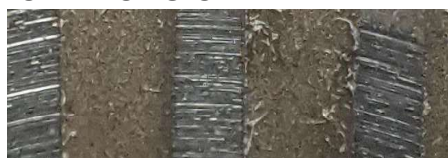
Photograph of an unfired insert showing grooves on the landings from machining.
