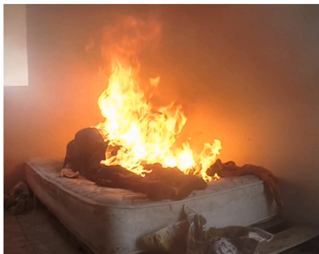
Fig. 6. Scene 2017/9 Bed ignited with flammable liquid.
