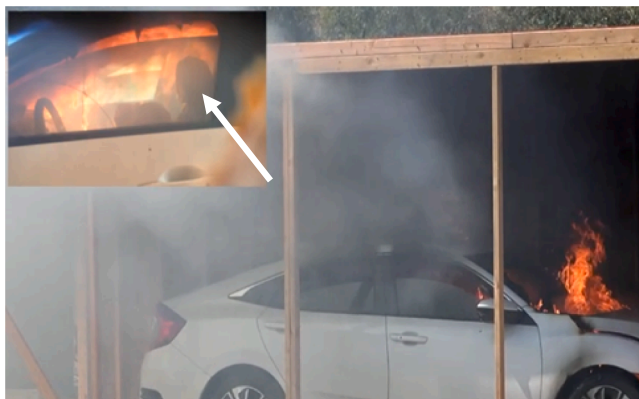
Fig. 12. Head in roof flame (indicated by arrow).
