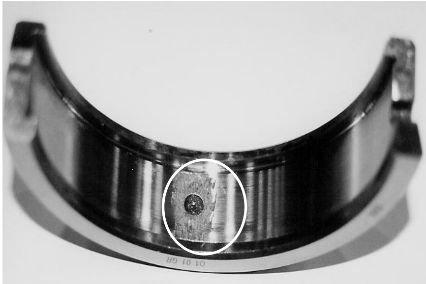
Figure 6 Rough defect condition
