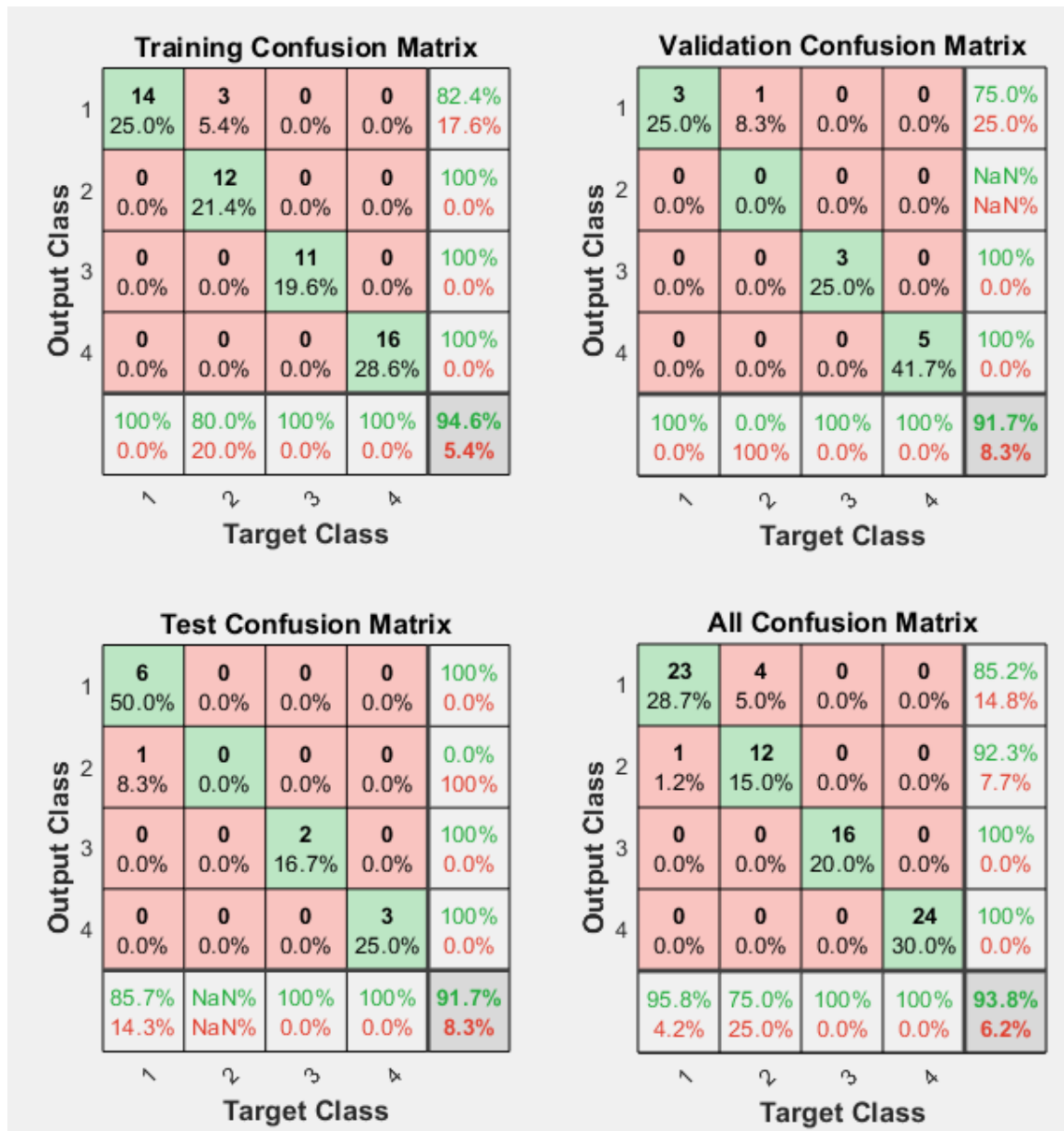
Figure 4-11. The confusion matrix of two-layer feed forward network used in damage assessment.
