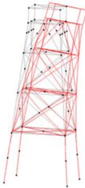
Figure 3-9b. Schematic of the finite element model of the fixed offshore platform used in this case study. (Karadeniz, 2001).
