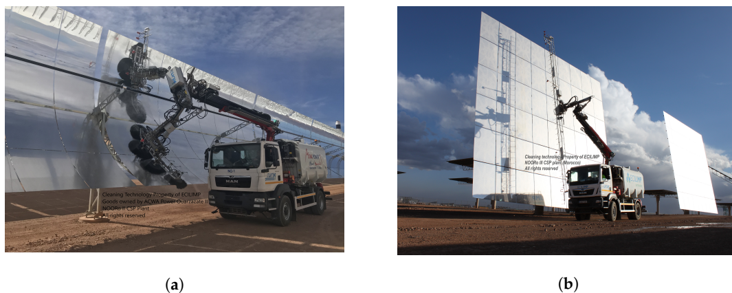
Figure 2. Semi-automatic cleaning in CSP plants (courtesy of ECILIMP Termosolar [23]). (a) Semi-automatic cleaning of parabolic troughs in Noor II; (b) Semi-automatic cleaning of heliostats in Noor III.
