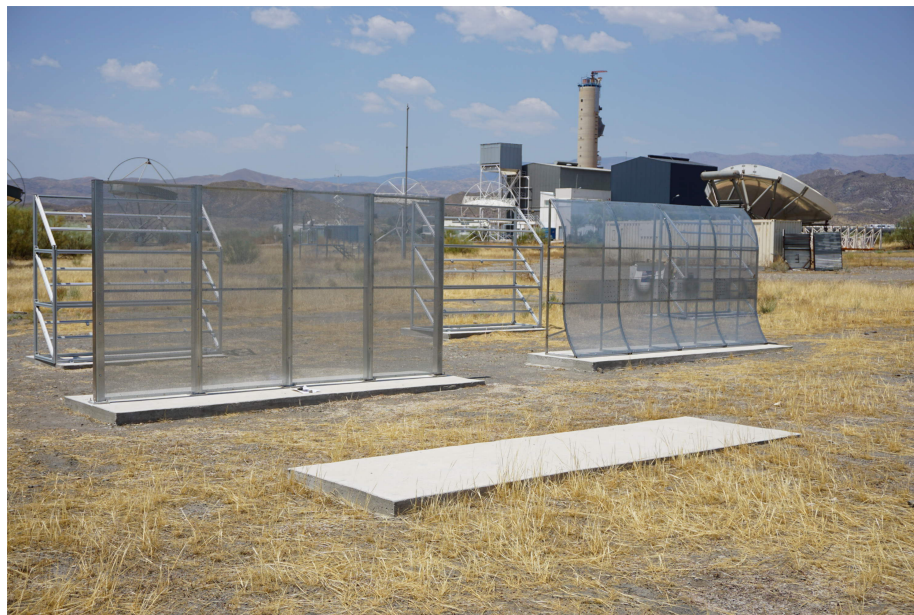
Figure 7. Dust barriers installed in PSA.
