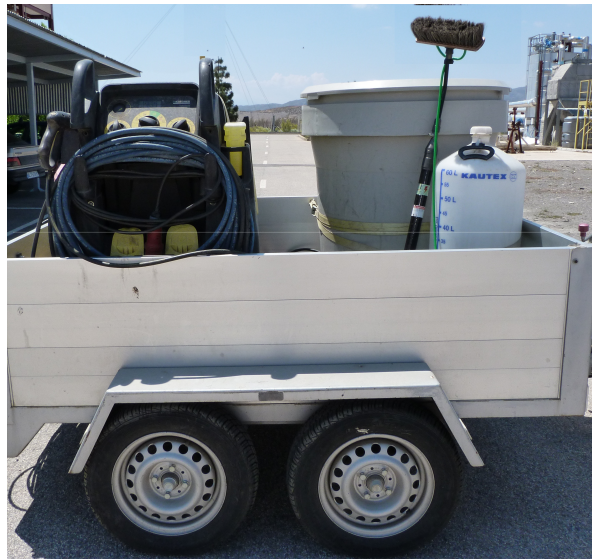
Figure 1. The set of cleaning tools used for washing exposed mirrors in PSA comprises high pressure nozzle, soft scrubbing brush, steam washer, tanks for both demineralized water and detergents [20].
