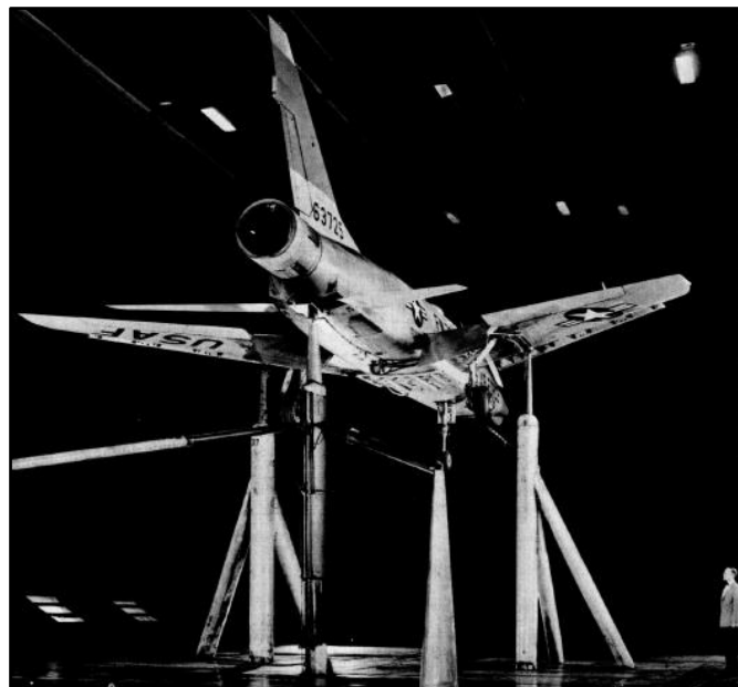
Figure 3.29: F-100F aircraft in the wind tunnel for cascade type thrust reverser testing. Image adopted from [Ref. 31].
