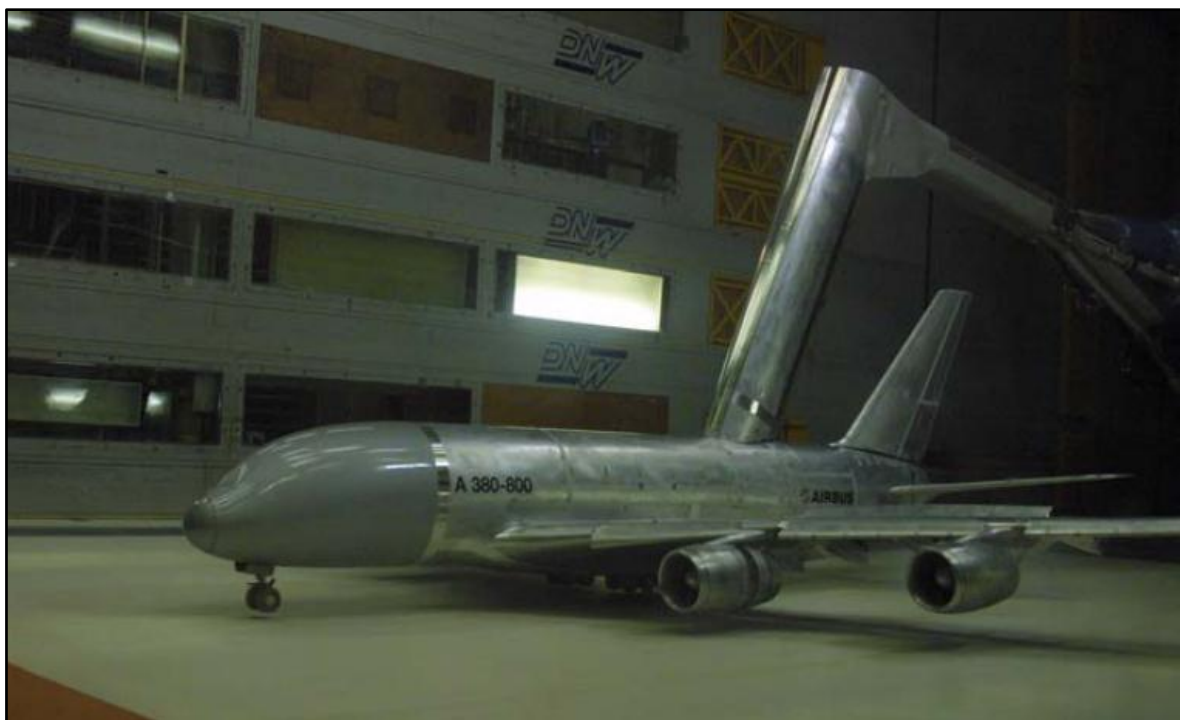
Figure 3.93: Dorsal sting supported Airbus A380 above the Moving Belt Ground Plane in DNW-LLF. Image adopted from [Ref. 49].
