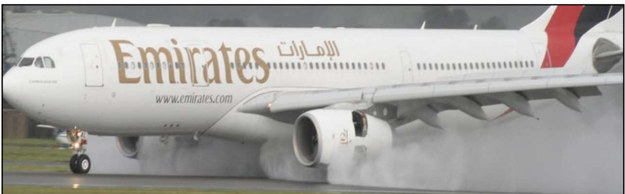
Figure 6.1: Deployed thrust reverser on a mixed exhaust engine. Reverser is operating only on fan stream flow. Images adopted from [Ref. 65].
