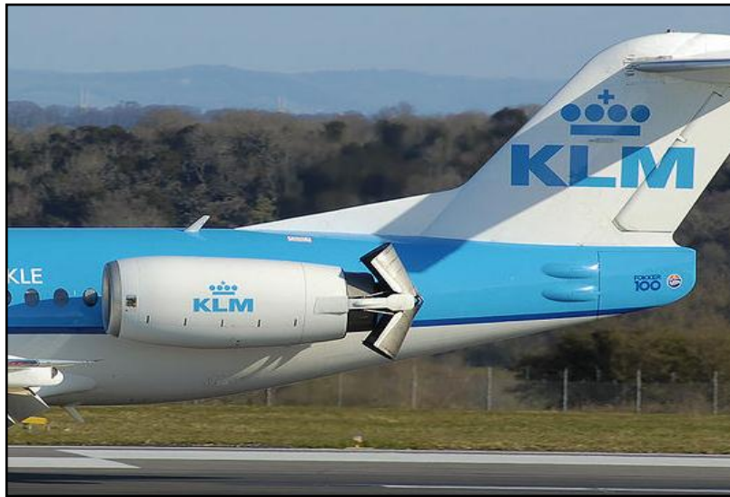
Figure 2.3: Target type thrust reverser in operation on Fokker aircraft. Images adopted from [Ref. 14].
