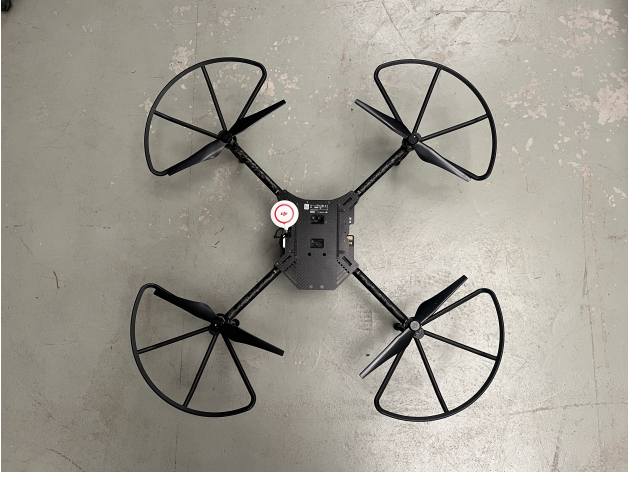
Fig. 3. DJI Matrice 100 used to collect measure data [36].
