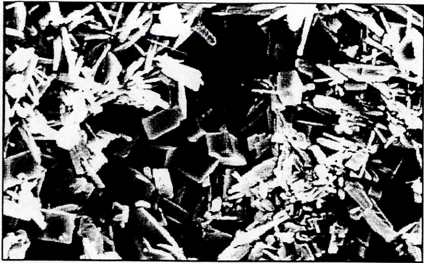
Figure 27: SEM picture of the interface between hard scale and soft scale layer
