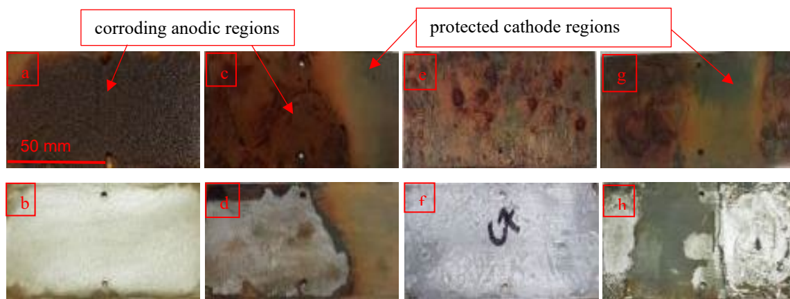
Figure 10 Pictorial view of the corroded and chemically cleaned steel coupons (C-series) collected from artificial seawater. Here exposure periods are as follows: (a, b) 45 days (c, d) 90 days (e, f) 210 days and (g, h) 321 days
