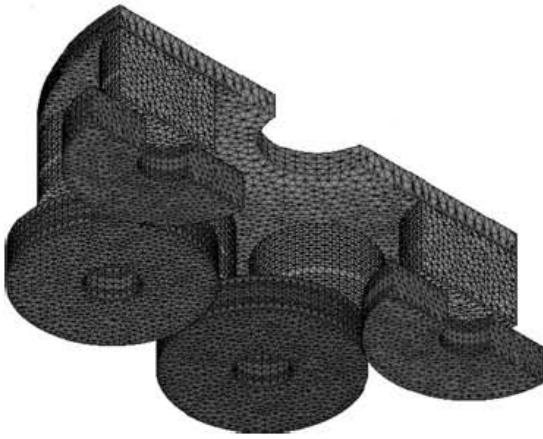
Figure 3 Meshed model of quarter of the machine
