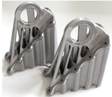
Figure 2-3: Airbus A350 XWB cabin bracket manufactured by SLM in Ti-6Al-4V. Note the net shape of the component and complexity of multiple features. Reproduced from [13].
