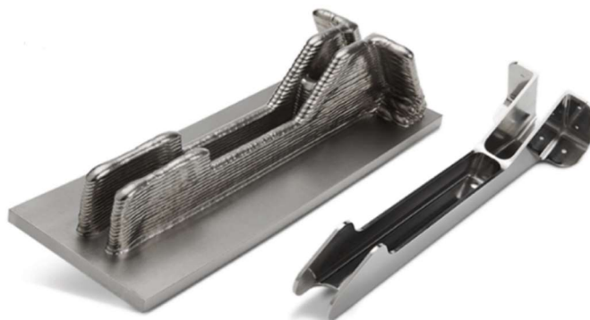
Figure 2-4: Example of Boeing 787 structural component deposited with WAAM using titanium (L) as-deposited (R) post-machining. Reproduced from [13].
