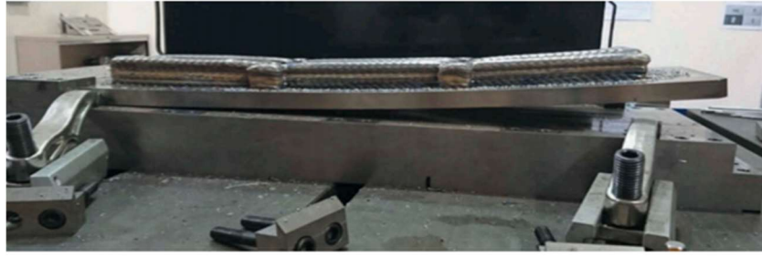
Figure 2-7: Distortion of Ti-6Al-4V cruciform deposit when unclamped due to residual stress accumulation. Reproduced from [174].
