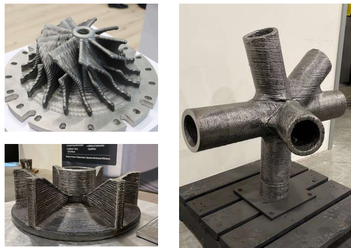
Figure 1-2: Examples of various complexity parts built using wire + arc additive manufacturing from steel and titanium [35,36].
