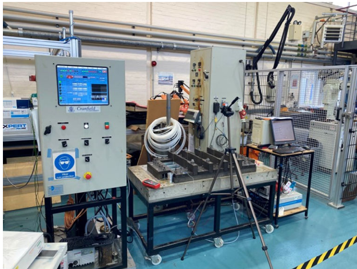
Figure 8. Experimental set-up used for glass top RTM trial.
