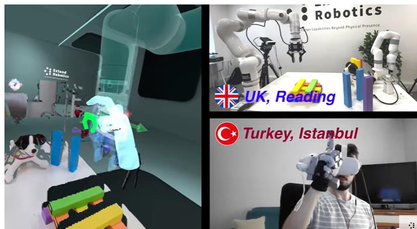
Figure 7-2 Extend Robotics low latency VR teleoperation demonstration between the UK and Turkey (October 2023)
