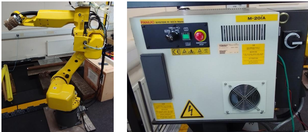
Figure 4-8 Fanuc M-20iA (left) and R-30iB mate cabinet (right)
