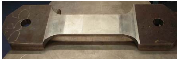
Fig. 1: BS EN 10025 Grade S275JR test specimen
