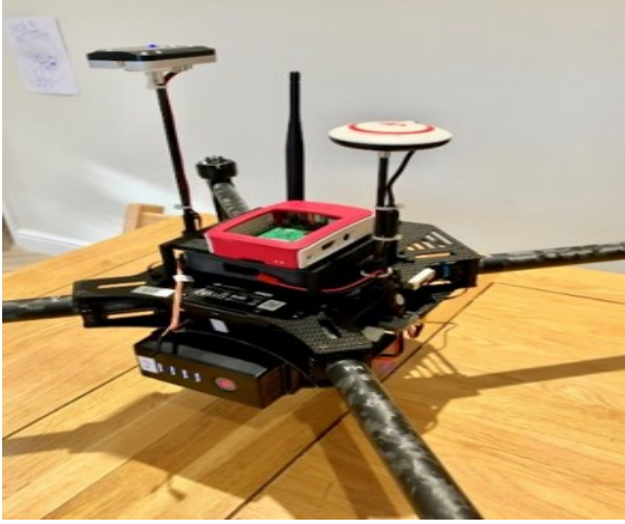
Fig. 11 DJI M100 with Raspberry-pi
