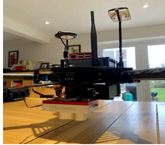
Fig. 12 DJI M100 with RedEdge and Xbee
