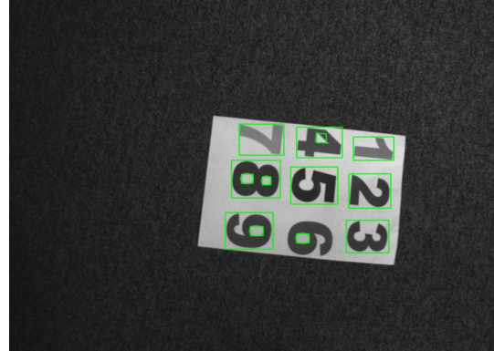
Fig. 7 Example of on-board image processing algorithm using KNN.
