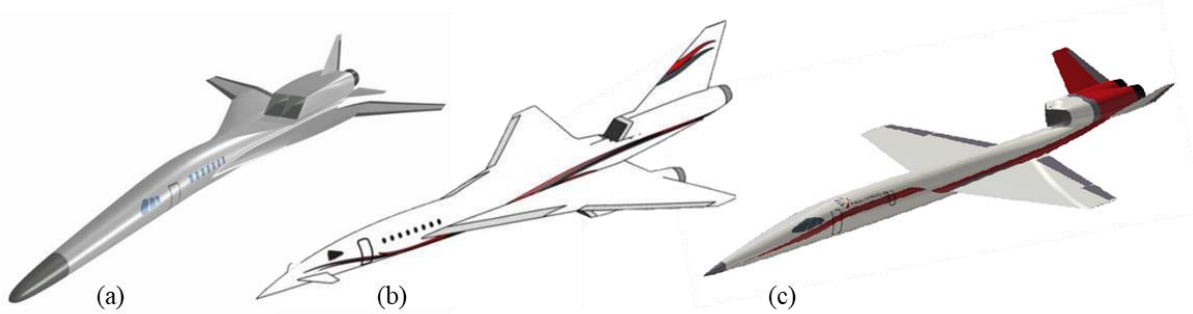
Fig. 1 External shape of low boom (a), low noise (b) and long range (c) HISAC concepts [1].
