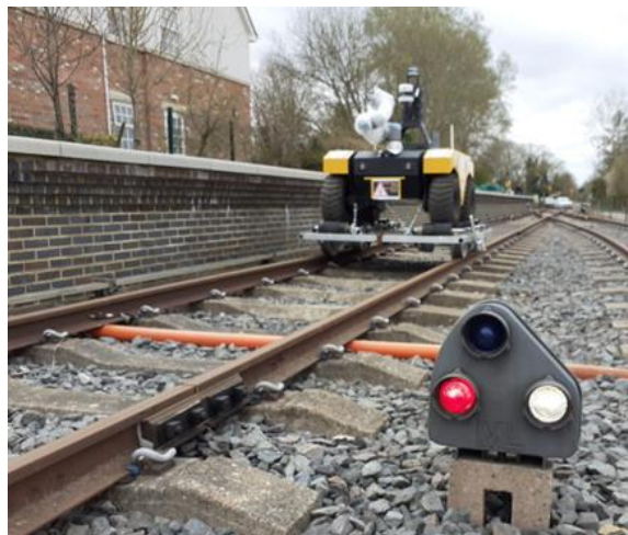
Figure 4-26 The robotic inspection and repair system (RIRS) on the Northampton & Lamport Railway
