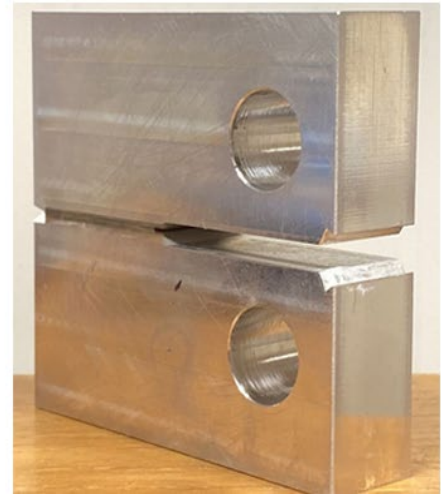
Fig. 2. Prepared CT specimens for fracture toughness test
