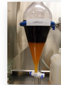
During sodium carbonate washing
