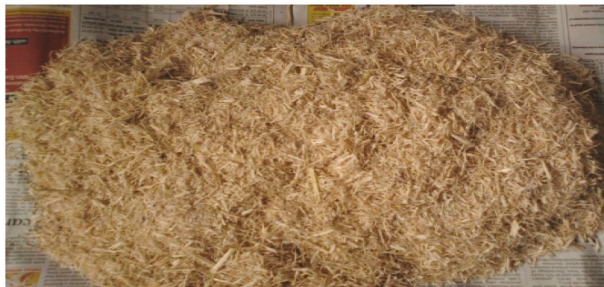
Figure 3. Chopped and treated sugarcane bagasse fibre.
