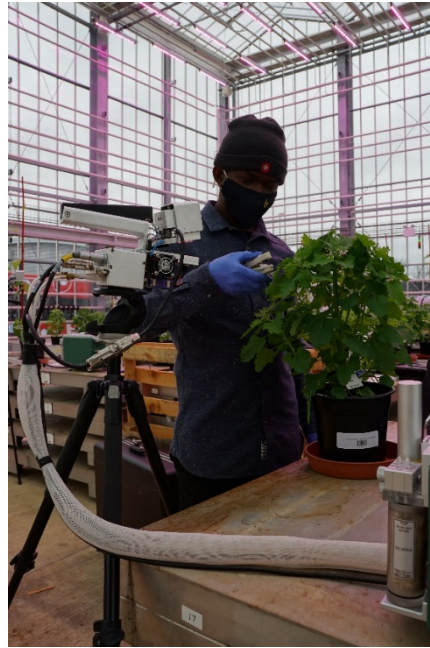
Figure B-2. The author taking gas exchange measurements for net CO 2 assimilation rate ( A_n ) using the portable photosynthetic system (Li-6400XT) along with SPAD measurement.
