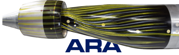
Figure 2.11: Photograph of an oil flow visualisation around the tail of a novel aircraft wind-tunnel model, courtesy of ARA
