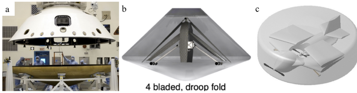
Fig. 6. a) Mars Science Laboratory aeroshell during testing (2011, size 4.5 m). Credits: NASA/Kim Shiflett. b) Folding option for coaxial helicopter concept in Pathfinder Aeroshell (size 2.65 m) [5]. c) Winged VTOL concept CAD model called FuMAD, folded and packed in Mars 2020 mission aeroshell (size 4.5) [37].
