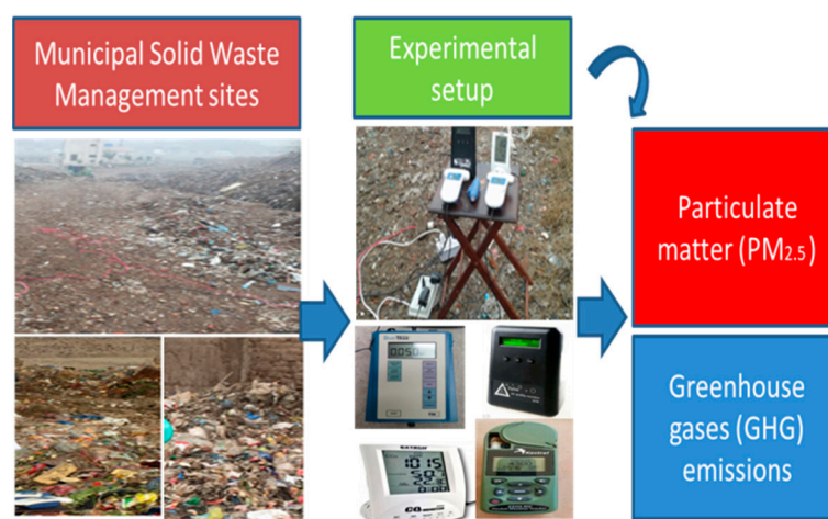
Figure 2. The conceptual diagram of experimental setup.
