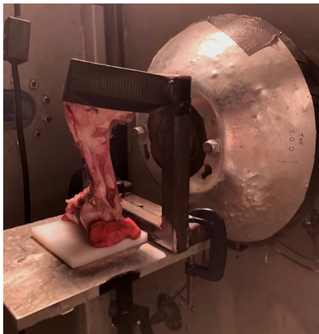
FIGURE 4 The experimental set-up of an individual femur on a stand inside of the gas gun target chamber in front of the muzzle of the gas gun, located on the right. The specially constructed ballistic stand is shown holding the femur upright in place.
