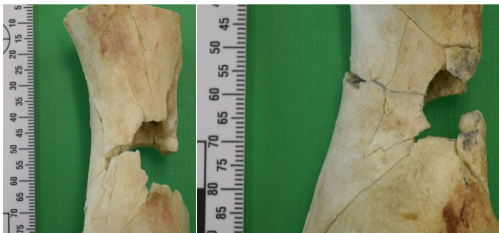
FIGURE 9 Left: a fractured femur impacted by a 0.357 JHP projectile in gel. Right: a fractured femur impacted by a 9 mm SJHP projectile in gel.
