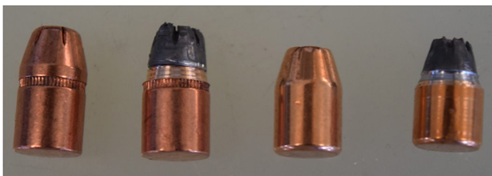
FIGURE 3 From left to right, a 0.357 JHP Hornady XTP® (10.2 g [30]), a 0.357 SJHP Hornady XTP® (9.8 g), a 9 mm JHP Sierra® (8.1 g [31]), and a 9 mm SJHP Sierra® (7.9 g) projectile.
