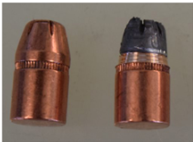
FIGURE 2 An HP bullet (left) and SJHP bullet (right) (image authors own).
