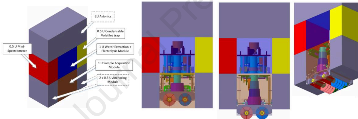
Figure 1-3 CAD representative of a 6U CubeSat concept and the internal system.
