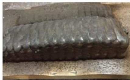
Fig. 8. Distortion during oscillation
