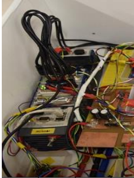
Figure 7-7 The NI Compact RIO system with input/output allocation
