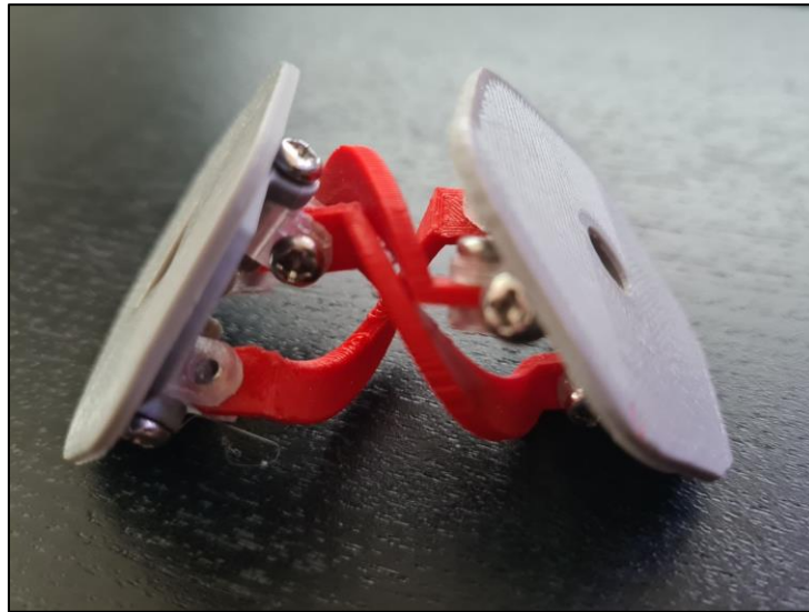
Figure 3.23. Prototype SASAR Quaternion Joint, showing Interfering limbs
