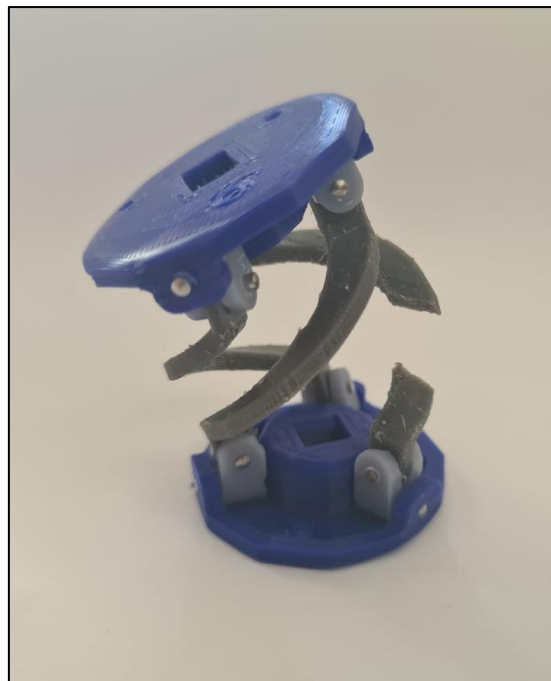
Figure 6.2. Example Quaternion Mechanism Showing Limb Failure
