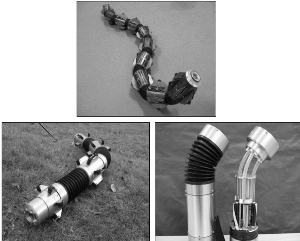
Figure 2.18: ACM-R5 (Top), ACM-S1 (Left), ACM-S1 Joint Mechanism (right) [74,75]
