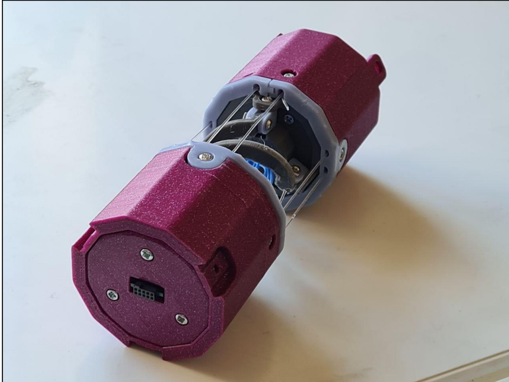
Figure 6.1. SASAR 2 Joint Module Showing Connection Interfaced
