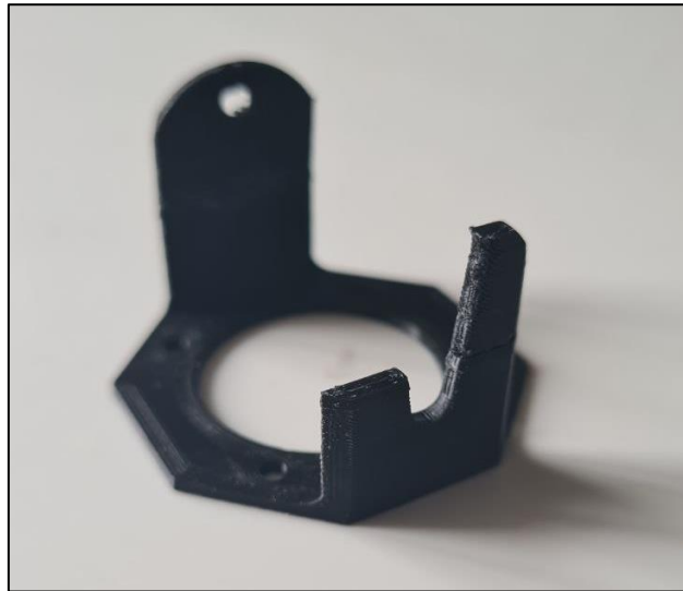
Figure 3.8. Prototype SASAR 1 Hinge Bracket Showing Layer Failure
