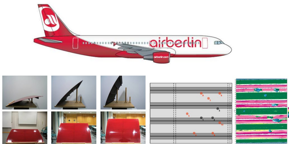
Figure 139. Effect of Painted Aircraft Livery on Composite Visual Inspections (87)
