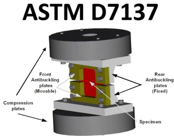
Figure 138. ASTM D7137 Test Specimen and Fixture Assembly Overview (86)
