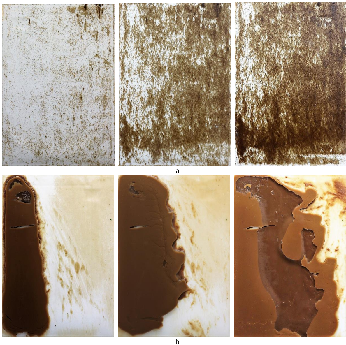
Figure 5: Examples of progressive sludging in 1-4 hour timeframe: (a) municipal, and (b) industrial MBR sludge sample, \text{MLSS} = 8\text{--}12\text{ g.L}^{-1} , U_a = 0\text{ m.s}^{-1} .
