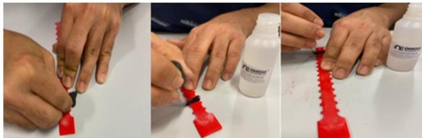
Applying the M-prep Conditioner, Neutralizer and scrubbing the surface using abrasive paper
