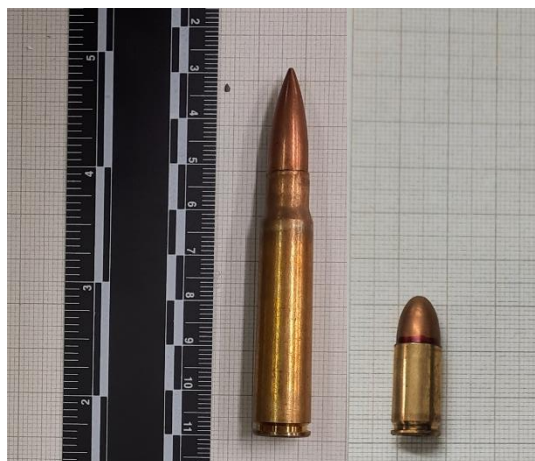
Figure 3 Photograph of ammunition used: 7.92x57 mm (left) and 9mm sk ptr m/39B (right)
