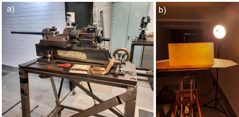
Figure 4 Photos of a) the proof mount with the Mauser barrel, b) the set-up of the gelatine block at the range
