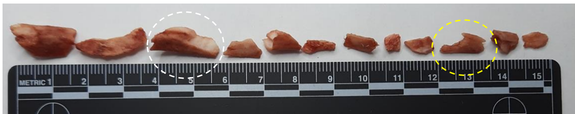
Figure 28 Photo of the overview of all fragments recovered after a rib (2.6) was shot with a 9mm projectile at 10m. The white circle indicates a fragment from the superior edge of the rib, and the yellow circle indicates a fragment from the inferior edge
