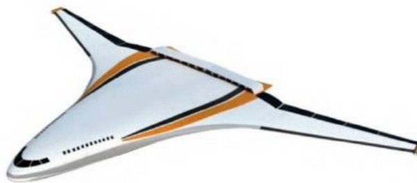
Figure 6 TeDP on a blended wing body airframe [47]
