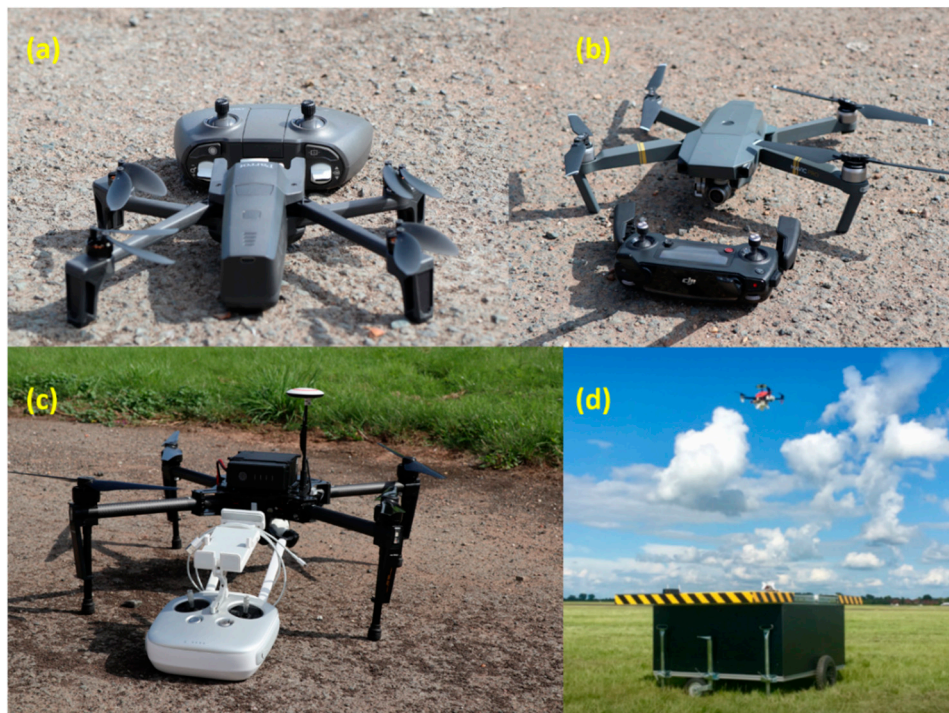
Figure 3. Unmanned aircraft systems compared for image quality acquisition at the Cranfield WWTP study site. (a) Parrot Anafi (Parrot, France); (b) DJI Mavic 2 Pro (DJI Technology Co, China); and (c) DJI Matrice 100 (DJI Technology Co, China). (d) Autonomous docking station (Herotech8, UK).
