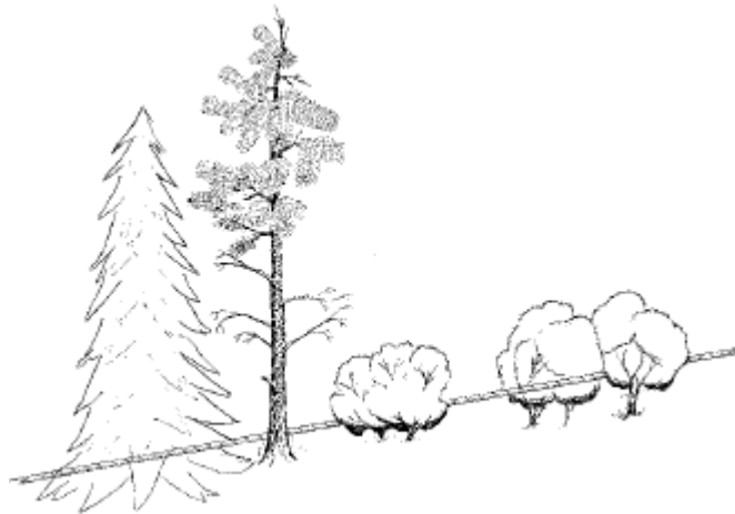
Figure 6. The measuring tape is stretched tight below, in or above the canopy vegetation , whatever position allows the easiest estimation of cover without zigzagging around plants.
