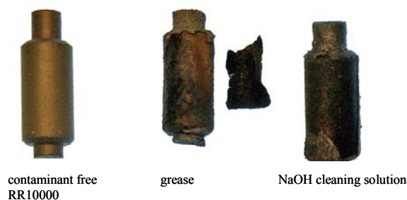
Figure 17. Appearance of samples exposed after 200 hours in air – 300 vpm SO 2 at 700°C (screening test).
