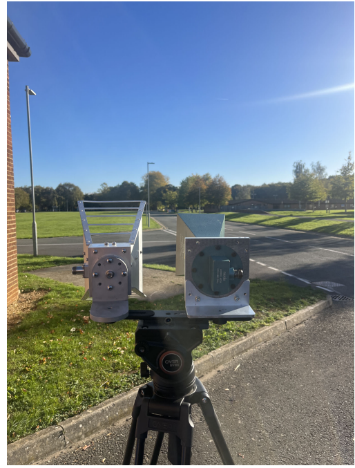
Fig. 19. Photo of the radar used to collect data with the antennas used to transmit and receive.
